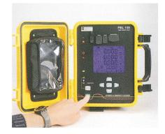
With its 1,000 V CAT IV safety rating, it can be used for measurements on all LV networks, including measurements of the neutral-earth voltage and the neutral current. This stand-alone instrument is equipped with a self-powering system via its voltage inputs up to 1,000 V. The PEL 105 offers 5 voltage inputs and 4 current inputs. Compatible with a large number of current sensors to make it easier to use, it also recognizes the sensors automatically.
