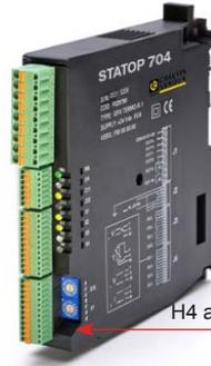
H4 and H6 LEDs are visible on the front side
